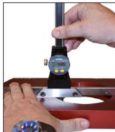
Depth measurement in a drilling with an additional base
