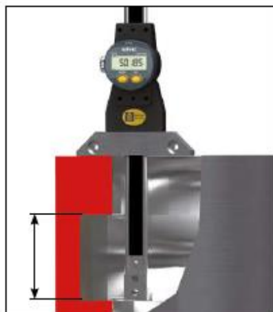
Measure of an internal groove (height) thanks to the constant.
